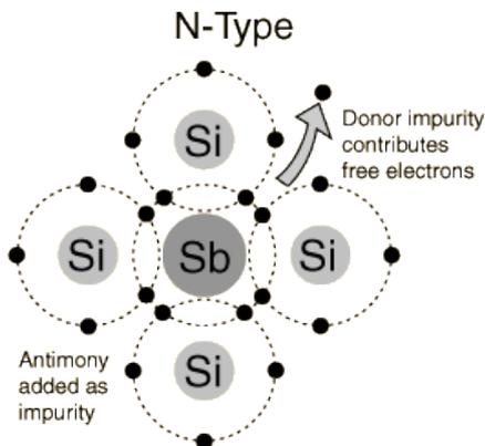
The addition of pentavalent impurities such as antimony, arsenic or phosphorous contributes free electrons, greatly increasing the conductivity of the intrinsic semiconductor. Phosphorous may be added by diffusion of phosphine gas ( $\text{PH}_3$ ).
