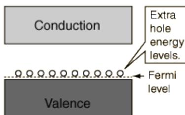
The addition of trivalent impurities such as boron, aluminum or gallium to an intrinsic semiconductor creates deficiencies of valence electrons, called "holes". It is typical to use  $\text{B}_2\text{H}_6$  diborane gas to diffuse boron into the silicon material.
