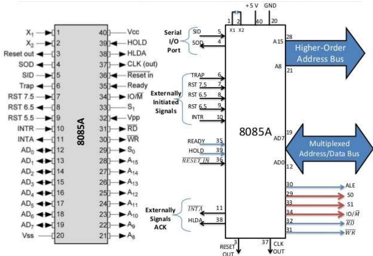
Fig 1.2 Pin Diagram of 8085A Microprocessor
