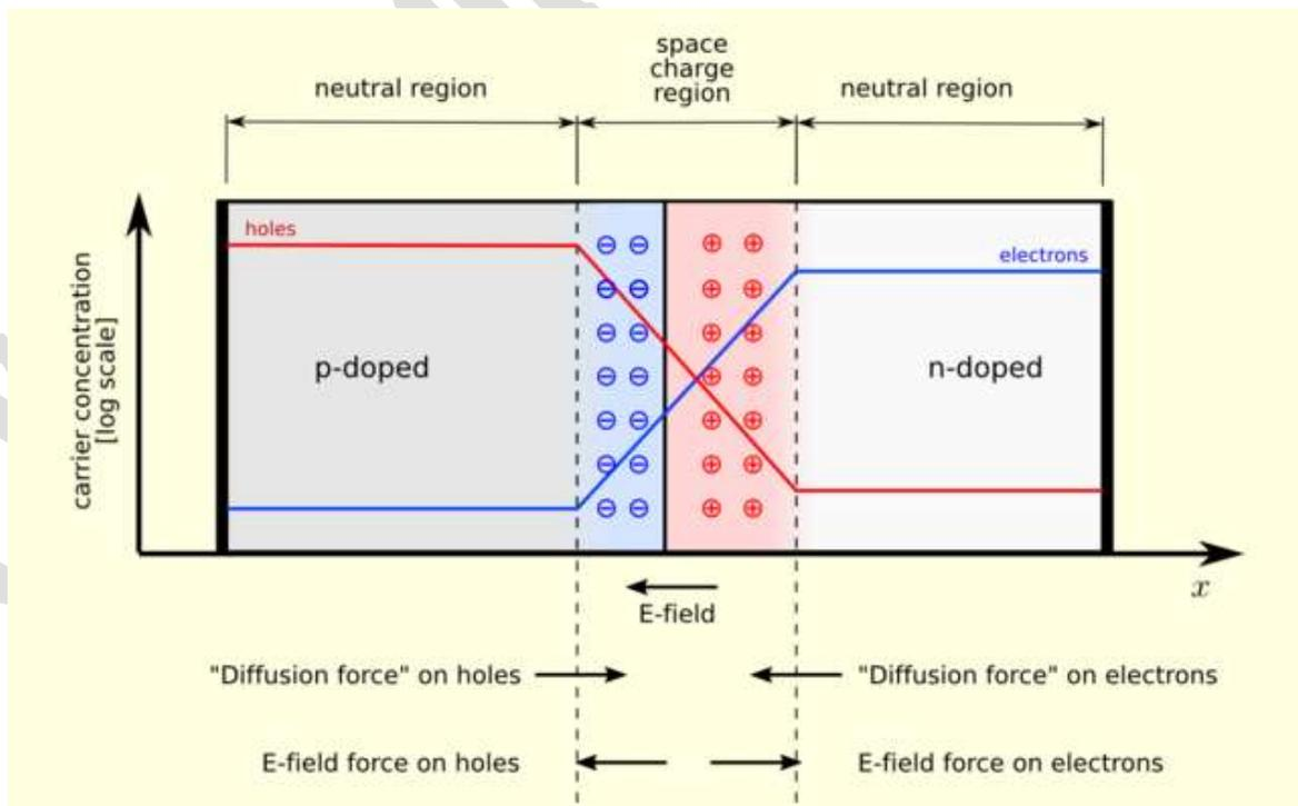
junctions are doped at a  $1e15/cm^3$  ( $0.00016C/cm^3$ ) doping level, leading to built-in potential of  $\sim 0.59$  V. Reducing depletion width can be inferred from the shrinking charge profile, as fewer dopants are exposed with increasing forward bias.
