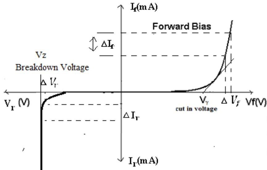
**Fig.1 V- I Characteristics of Zener Diode under Forward & Reverse Bias Conditions**
